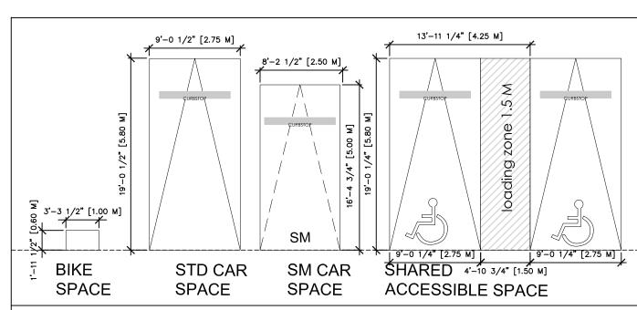
DIMENSIONS OF CAR AND BIKE PARKING SPACES USED IN THIS PROJECT
